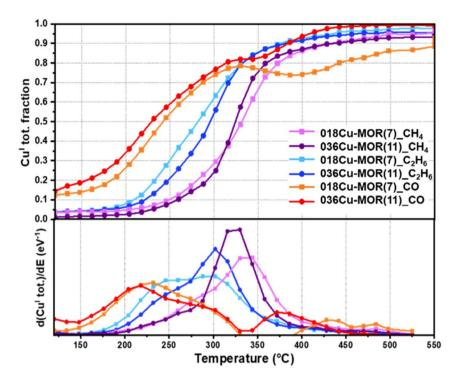
Fig. 3 Comparison of MCR-derived total  $Cu^{I}$  fraction as a function of temperature for each sample/reactant combination (top panel) in the  $CH_{4}$ -,  $C_{2}H_{6}$ -, and CO-TPR steps, and corresponding first derivative (bottom panel) to better identify inflection points in the  $Cu^{I}$  total fraction profile.
