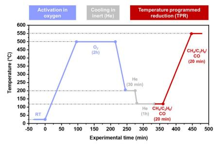
Scheme 1 Experimental protocol for *in situ* XAS during TPR experiments over Cu-MOR samples. The protocol consists of activation in oxygen at 500 °C, followed by two cooling steps. First, the sample was cooled in oxygen until 200 °C before a second cooling step to 120 °C in inert (He). Then the samples were exposed to a reductive atmosphere (either CH<sub>4</sub>, C<sub>2</sub>H<sub>6</sub>, or CO) while the temperature was ramped up (5 °C min<sup>-1</sup>) to 550 °C.
