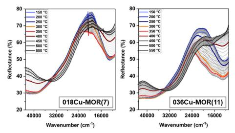
Fig. 5 In situ UV-vis spectra were obtained during a TPR protocol with  $CH_4$  for the two Cu-MOR samples. The spectra are overlayed, with a thick line, and different colors are used for every 50 °C to clarify the change in the spectra throughout the protocol. Blue colors are for low temperatures, red for intermediate temperatures, and dark grey for high temperatures.
