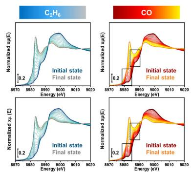
Fig. 1 XANES TPR spectra for each sample/reducing agent combination. The temperature was ramped up (5 °C min<sup>-1</sup>) from 120 °C to 550 °C for 1.5 h. The increased intensity of the rising edge 1s  $\rightarrow$  4p peak related to Cu<sup>I</sup> observed in all spectra, indicates the progressive formation of Cu<sup>I</sup> species during the TPR experiments. A more complex situation is visible in the case of CO, in which an intermediate Cu<sup>I</sup> species is detected (black boxes).
