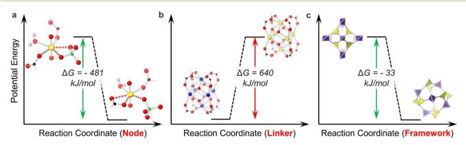
Fig. 1 Thermodynamic favorability of (a) ligand motifs in ref. 53: URCP3 on the left and URCP4 on the right. Bonds of interest are dashed; (b) node motifs in ref. 55:  $Zr_6$  cluster on the left and  $U_6$  cluster on the right; (c) framework topologies in U-MOFs in ref. 57: NU-1306 on the left and NU-1305 on the right. O is shown in red, U in yellow, C in black, H in pink, S in green, and Zr in blue.
