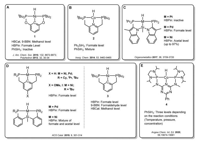
Fig. 2 Selected examples of pincer complexes for the catalytic hydroboration and hydrosilylation of CO<sub>2</sub>.
