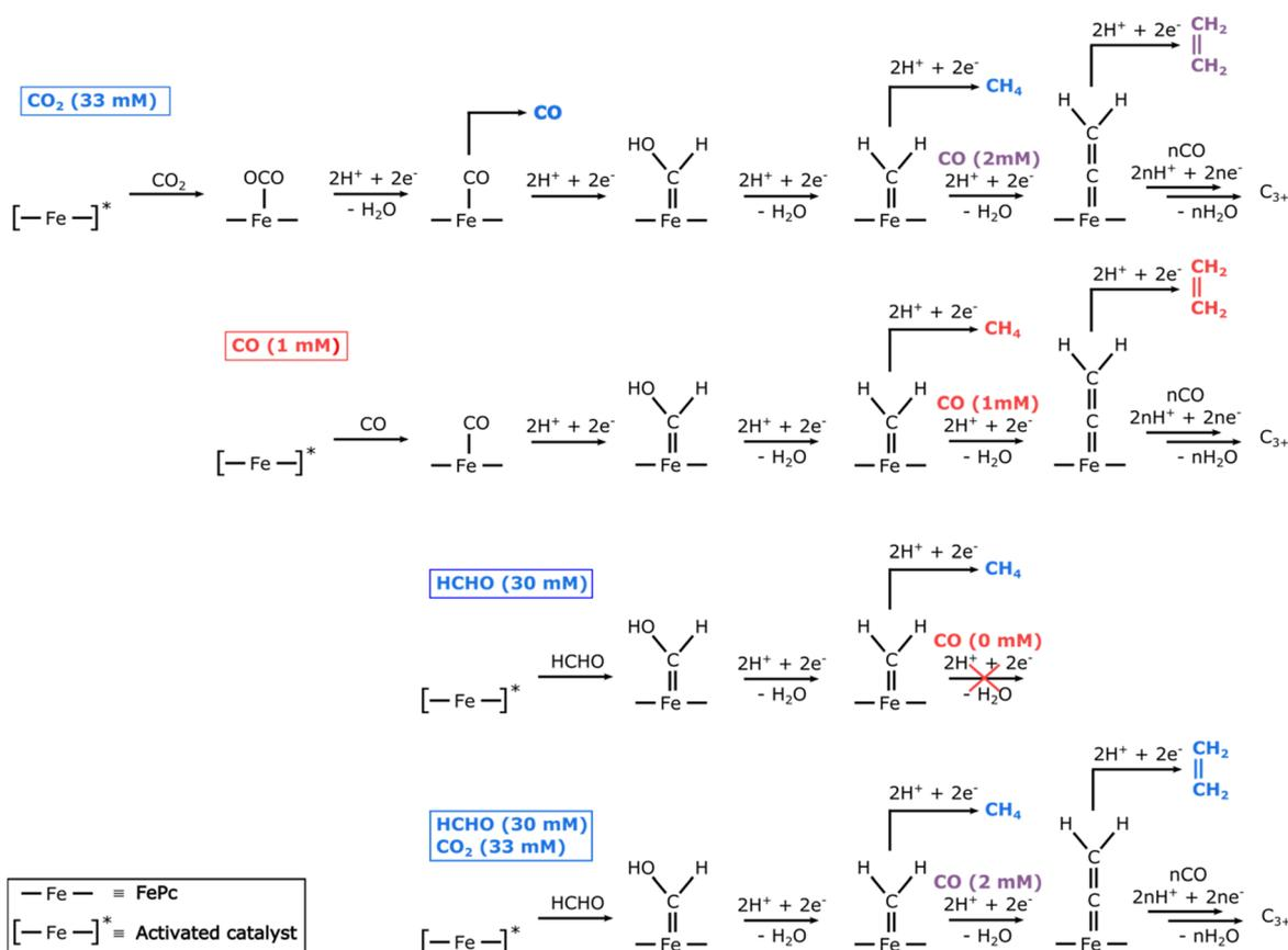
Fig. 6 Simplified mechanisms proposed for the formation of C–C bonds by FePc with either CO<sub>2</sub>, CO, HCHO, or a mixture of HCHO and CO<sub>2</sub> as substrates. The colour code for substrates and products is as follow: blue, purple, and red for high, intermediate, and low concentrations, respectively.
