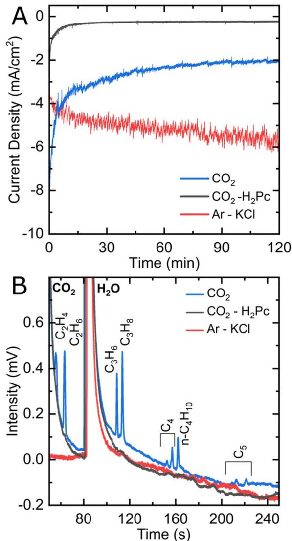
Fig. 2 (A) Chronoamperometric curves and (B) module B gas chromatograms of FePc-modified electrodes under Ar in 0.1 M KCl (red) and CO<sub>2</sub> in 0.1 M KHCO<sub>3</sub> (blue) and an H<sub>2</sub>Pc-modified electrode under CO<sub>2</sub> in KHCO<sub>3</sub> (black). Chronoamperometric experiments are performed at -1.1 V vs. RHE for two hours, after which a gas chromatograph (GC) samples their resulting gaseous products.
