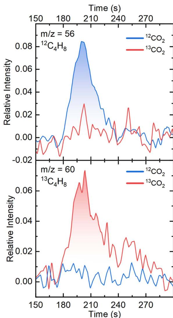
Fig. 3 GC-MS chromatograms for mass  $m/z = 56$  of  $^{12}\text{C}_4\text{H}_8$  and mass  $m/z = 60$  of  $^{13}\text{C}_4\text{H}_8$  at the retention time of  $\text{C}_4$  products. Chronoamperometric experiments were performed on FePc-modified electrodes at  $-1.1$  V vs. RHE for two hours, after which the GC-MS sampled the resulting gaseous products. The chromatograms were averaged from three independent experiments.
