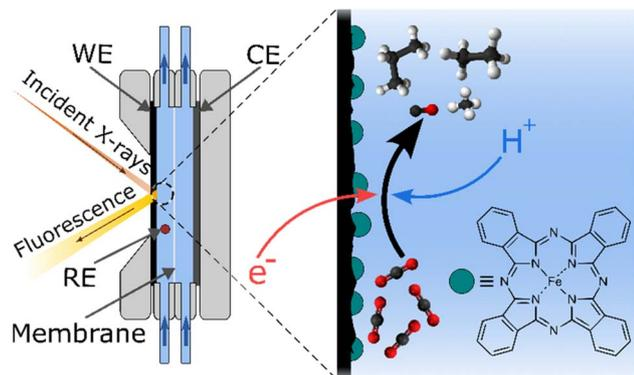
Fig. 1 Schematic side view of the electrochemical cell and simplified CO<sub>2</sub> reduction process on the surface of the working electrode. The dark green circles represent iron phthalocyanine (FePc), the molecular catalyst used in this study, whose structure is shown in the right corner. WE, CE, and RE stand for "working electrode", "counter electrode", and "reference electrode", respectively. The scheme is not drawn to scale.
