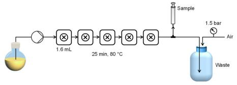
Fig. 1 Reactor platform for polymer synthesis in a miniature five-CSTR cascade. All five reactors are heated from the same temperature-controlled heating block, with stirring provided by five pairs of neodymium magnets glued to 5 V DC computer fans located underneath the heating block.
