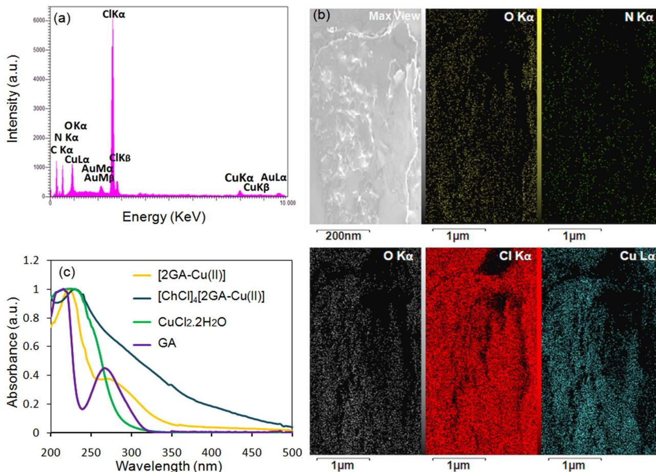
Fig. 4 (a) EDX analysis; (b) mapping images of the constructing elements of [ChCl]<sub>4</sub>[2GA-Cu(II)]; (c) UV-Vis normalized spectra of CuCl<sub>2</sub>·2H<sub>2</sub>O, GA, [2GA-Cu(II)], and [ChCl]<sub>4</sub>[2GA-Cu(II)] in deionized water (0.0005 M).
