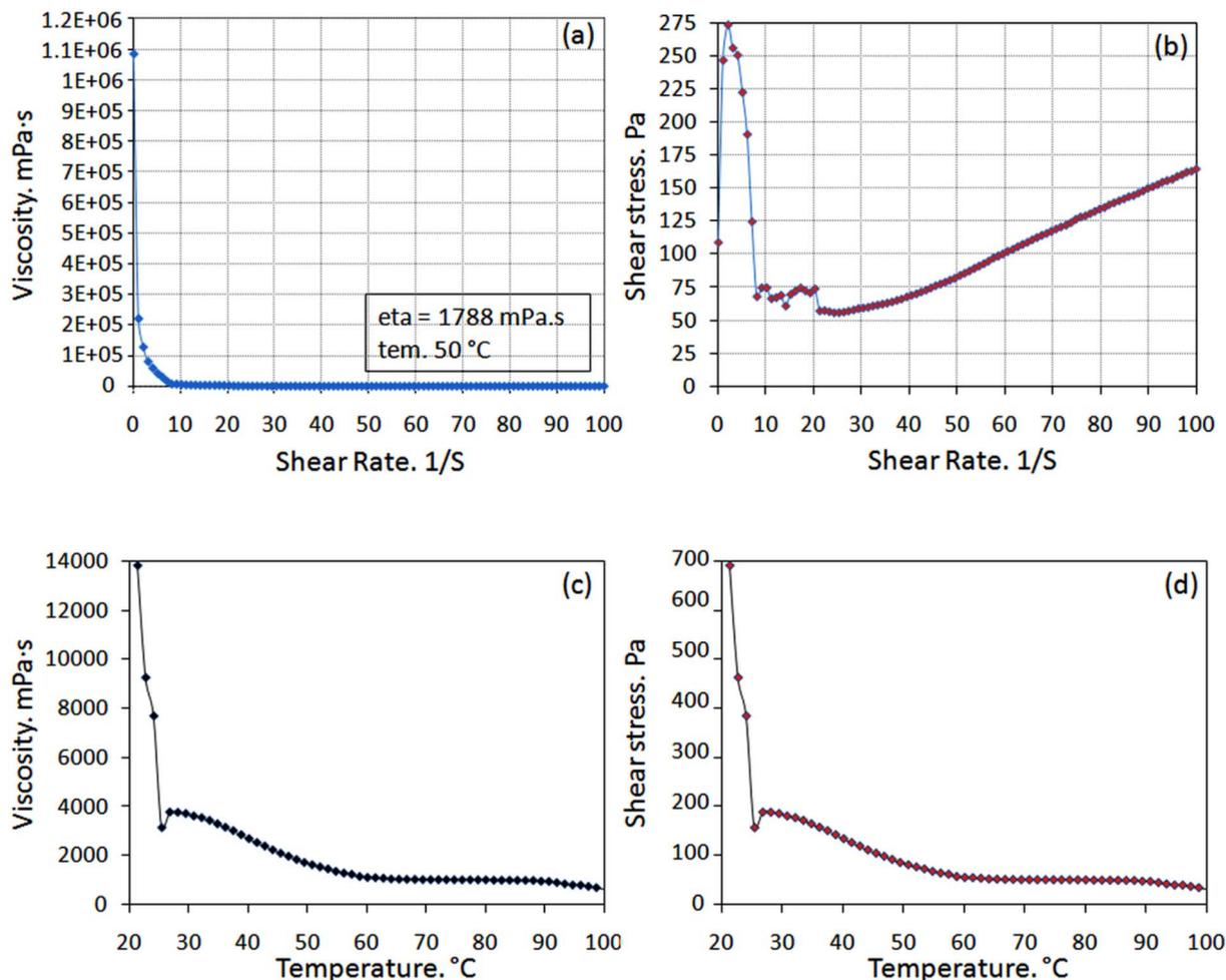
Fig. 5 (a) Viscosity versus shear rate at 50 °C and (b) shear stress versus shear rate at 50 °C of  $[\text{ChCl}]_4[2\text{GA-Cu(II)}]$ ; (c) dependence viscosity versus temperature, and (d) dependence shear stress versus temperature at shear rate  $50 \text{ s}^{-1}$  of  $[\text{ChCl}]_4[2\text{GA-Cu(II)}]$ .
