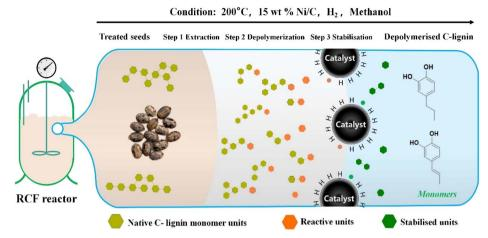
Fig. 4 Reductive catalytic fractionation (RCF) process of C-lignin.<sup>16</sup>
