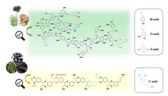
Fig. 1 Proposed structure of H/G/S lignin versus C-lignin revealed by NMR analysis.<sup>15</sup>
