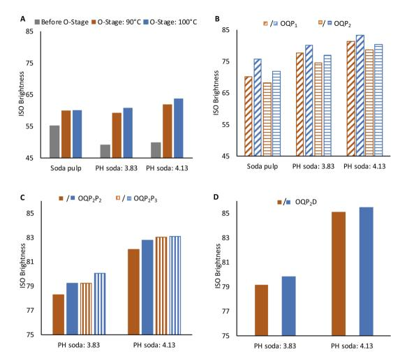
Fig. 4 ISO brightness of pulps before and after oxygen (O) bleaching (A) after  $OQP_1$  and  $OQP_2$  (B), after  $OQP_2P_2$  and  $OQP_2P_3$  (C) and after  $OQP_2D$  (D) (temperature of O-stage in the sequences are indicated by  $\blacksquare$  for 90 °C and  $\blacksquare$  for 100 °C).
