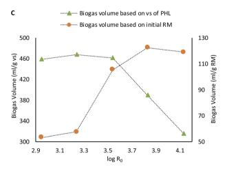
Fig. 5 Effect of steaming severity on acetic acid content and pH of PHL (A) on carbohydrate and furan content of PHL (B) and on BMP of PHL based on volatile solid (vs.) and raw material (RM) (C).
