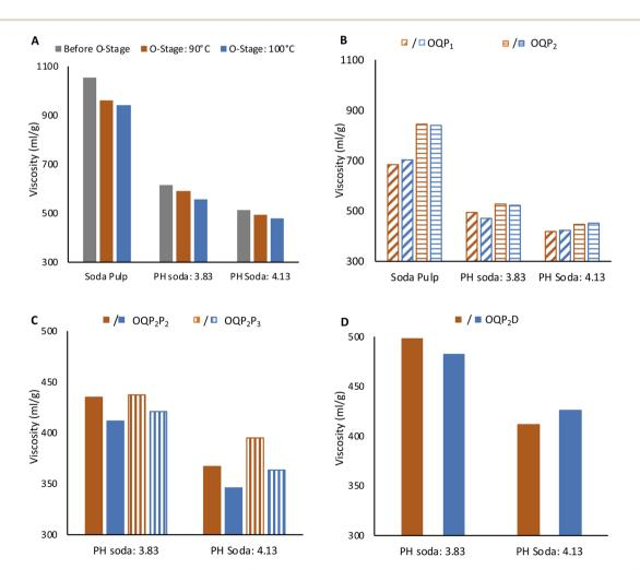
Fig. 3 CUEN viscosity of pulps before and after oxygen (O) bleaching (A) after  $OQP_2$  and  $OQP_2$  (B), after  $OQP_2P_2$  and  $OQP_2P_3$  (C) and after  $OQP_2D$  (D) (temperature of O-stage in the sequences are indicated by  $\blacksquare$  for 90 °C and  $\blacksquare$  for 100 °C).
