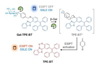
Fig. 1 Schematic illustration of the ratiometric detection of β-galactosidase based on excited-state intramolecular proton transfer (ESIPT) and solid-state luminescence enhancement (SSLE).
