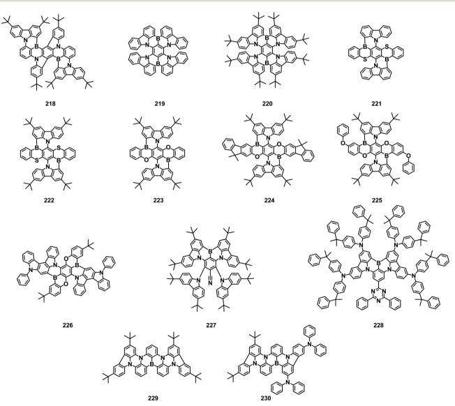
Fig. 6 Molecular structures of red B/N-based TADF emitters containing DABNA units.
