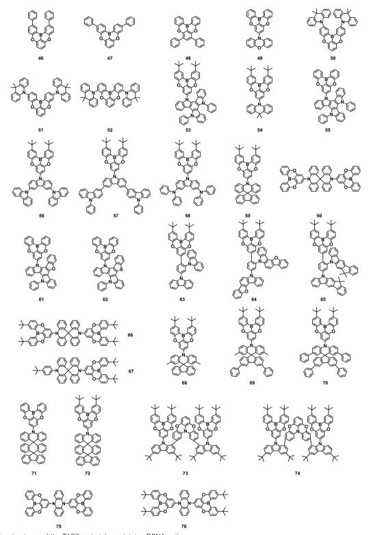
Fig. 3 Molecular structures of the TADF materials containing DBNA units.
