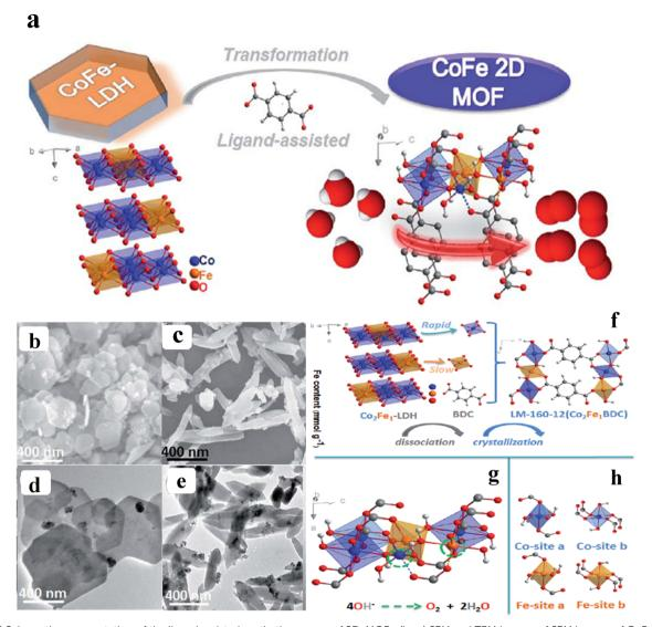
Fig. 2 (a) Schematic representation of the ligand assisted synthetic process of 2D-MOFs. (b-e) SEM and TEM images of SEM images of CoFe-LDH and LM-160-12; (f) The graphic representation of the structural change from LDHs to 2D MOFs; (g) The local unsaturated model (green dashed circle) for the metals on LM-160-surface 12's; (h) Four different pairs of [MO<sub>6</sub>] octahedra. Reprinted with permission from ref. 48. Copyright (2020) Royal Society of Chemistry (RSC).
