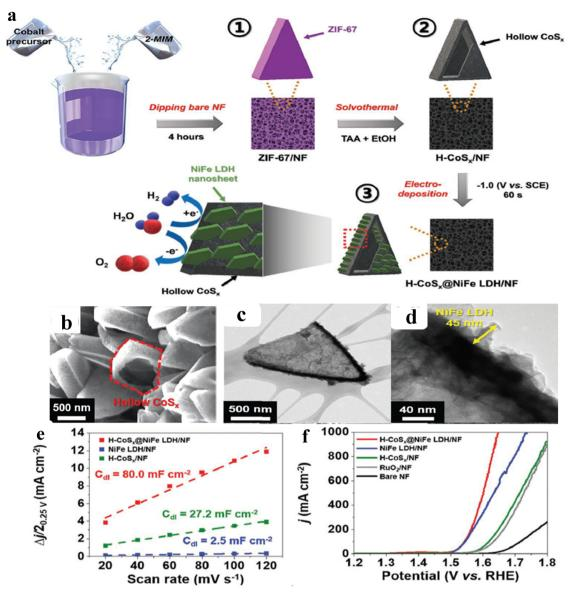
Fig. 14 (a) Schematic diagram of the fabrication process of H-CoS<sub>x</sub>@NiFe LDH/NF; (b) SEM images of H-CoS<sub>x</sub>/NF; (c and d) TEM and HR-TEM images of  $H-CoS_x/NF$ ; (e) calculated  $C_{al}$  values at current densities vs. scan rates; (f) OER performance of all the catalysts at 1 M KOH solution. Reprinted with permission from ref. 96. Copyright (2022) Wiley-VCH.
