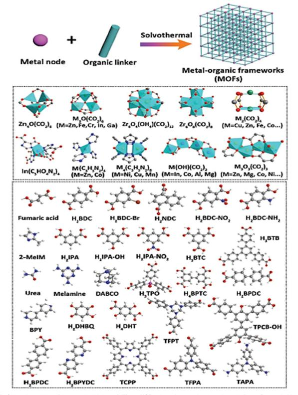
Scheme 1 Schematic depiction of the theoretical designs of different MOFs using various metal nodes and organic linkers. Reprinted with permission from ref. 21. Copyright (2021) Wiley-VCH.
