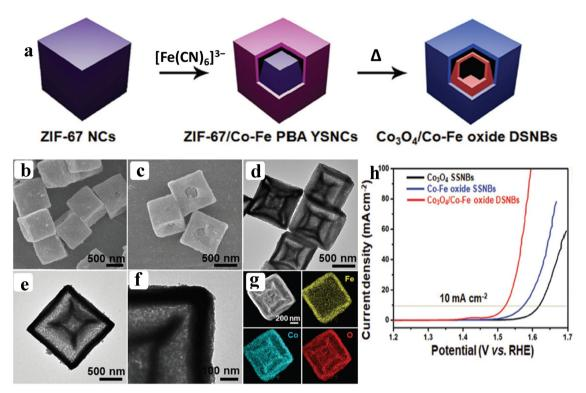
Fig. 9 (a) Schematic representation of the formation process of  $Co_3O_4/Co$ -Fe oxide DSNBs; (b and c) and (d-f) show the FE-SEM and HR-TEM images of Co<sub>3</sub>O<sub>4</sub>/Co-Fe oxide DSNBs, respectively; (g) corresponding HAADF elemental mapping results; (h) LSV outcomes of Co<sub>3</sub>O<sub>4</sub>/Co-Fe oxide DSNBs, Co-Fe oxide SSNBs, and Co<sub>3</sub>O<sub>4</sub> SSNBs. Reprinted with permission from ref. 72. Copyright (2018) Wiley-VCH.
