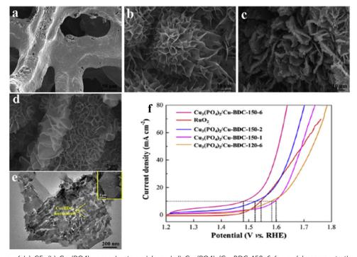
Fig. 8 FESEM images of (a) CF, (b) Cu<sub>3</sub>(PO4)<sub>2</sub> nanosheets and (c and d) Cu<sub>3</sub>(PO4)<sub>2</sub>/Cu-BDC-150-6 foam; (e) represents the HR-TEM images of Cu<sub>3</sub>(PO4)<sub>2</sub>/Cu-BDC; (f) LSV polarization results of Cu<sub>3</sub>(PO4)<sub>2</sub>/Cu-BDC foams and commercial RuO<sub>2</sub>. Reprinted with permission from ref. 66. Copyright (2019) Elsevier.
