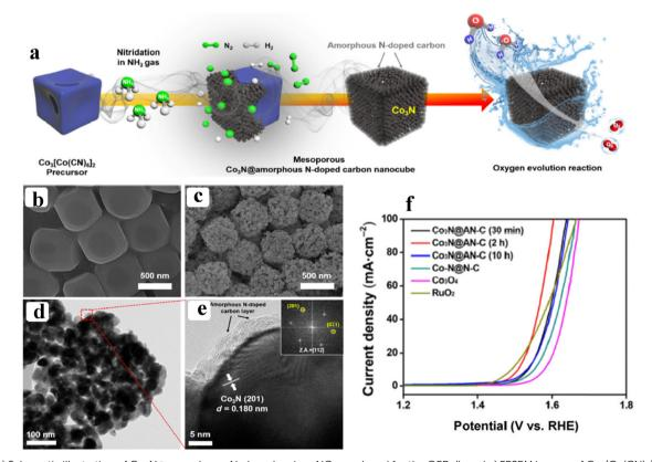
Fig. 16 (a) Schematic illustration of Co<sub>x</sub>N@amorphours N-doped carbon NCs employed for the OER; (b and c) FESEM images of Co<sub>x</sub>(Co(CN)<sub>6</sub>)<sub>2</sub> PBA and Co<sub>3</sub>N@AN-C NCs; (d and e) TEM and HR-TEM images of Co<sub>3</sub>N@AN-C NCs (inset image is FFT patterns); (f) IR corrected LSV polarization curves of Co<sub>3</sub>N@AN-C NCs, Co-N@N-C, and Co<sub>3</sub>O<sub>4</sub> NCs. Reprinted with permission from ref. 103. Copyright (2019) Springer.
