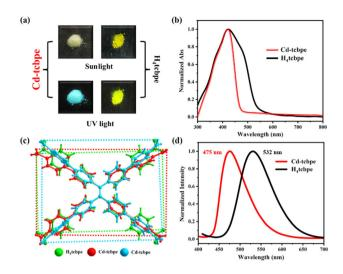
Fig. 2 (a) Emissive photographs of Cd-tcbpe and H<sub>4</sub>tcbpe under a hand UV light of 365 nm; (b) UV-vis spectra of Cd-tcbpe-B and H<sub>4</sub>tcbpe ligand; (c) comparison of tcbpe linkers in Cd-tcbpe (red, blue) and  $H_4$ tcbpe (green); (d) fluorescence emission spectra of **Cd-tcbpe** ( $\lambda_{ex}$  = 370 nm) and H<sub>4</sub>tcbpe ( $\lambda_{ex}$  = 390 nm).
