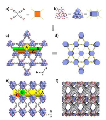
Fig. 1 (a and b) The 4-c TCPE<sup>4-</sup> ligand and the 12-c nonanuclear Tb<sub>9</sub> cluster. (c and e) The 3D framework of NKU-200-Tb with three types of 1D channels along the c- and a-axis, respectively. (d) The topological simplification of the (4,12)-c shp net. (f) View of channels B and C in the Connolly surface.
