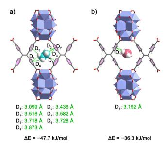
Fig. 4 (a and b) Predicted adsorption sites, interactions, and binding energies ( $\Delta E$ ) of C<sub>2</sub>H<sub>6</sub> and C<sub>2</sub>H<sub>4</sub> in the nanotrap of NKU-200-Tb obtained from the DFT optimization. The green dashed lines refer to C- $H \cdots \pi$  interactions
