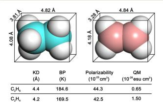
**Scheme 1** Molecular structure and physical properties of  $C_2H_6$  and  $C_2H_4$ , KD = kinetic diameter. BP = boiling point, QM = quadrupole moment.
