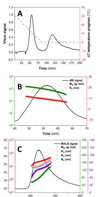
Fig. 5 ThFFF results for SCNP-shell nanostructures of PS $_{102}$ -PEO $_{34}$  at a  $\Delta T$  of 30 °C for 1 min elution time, with a programmed linear temperature decay to 0 °C over 80 min, at a flow of 0.1 mL min $^{-1}$ : the parameters are recorded vs.  $T_R$  as follows: (A)  $\Delta T$  temperature program across the Visco signal;  $R_G$ ,  $R_V$  and  $R_H$  distributions overlaid on the MALS signal for: (B) SCNP-shell and (C) MCNP nanostructures.
