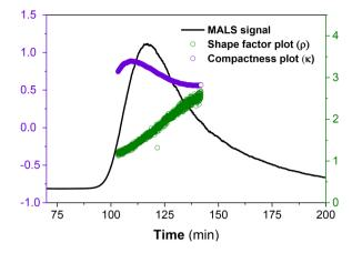
**Fig. 6** Shape factor  $(\rho)$  and compactness  $(\kappa)$  plots for PS<sub>102</sub>-PEO<sub>34</sub> MCNP nanostructures at a  $\Delta T$  of 30 °C for 1 min elution time, with a programmed linear temperature decay to 0 °C over 80 min, at a flow of 0.1 mL min<sup>-1</sup>.
