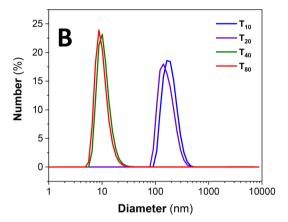
Fig. 3 Size dynamics for  $PS_{102}$ – $PEO_{34}$  as a function of temperature (A) by intensity % and (B) number %; where the subscripts represent the measurement temperature in °C.
