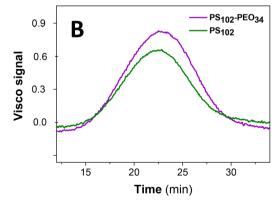
Fig. 1 (A) DLS measurement of  $PS_{102}$ – $PEO_{34}$  in toluene (selective solvent) and chloroform (good solvent) at 25 °C; (B) ThFFF elution behaviour of  $PS_{102}$  homopolymer vs.  $PS_{102}$ – $PEO_{34}$  having a PS block of comparable size to that of the PS homopolymer. Solvent: toluene; temperature gradient: ΔT 60 °C; flow: 0.4 mL min<sup>-1</sup>.
