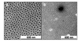
Fig. 2 TEM micrographs for PS<sub>102</sub>-PEO<sub>34</sub> nanostructures: SCNP-shell (A); SCNP-shell and dense sphere-like MCNPs (B). All samples were stored and cooled in a fridge at 7 °C prior to analysis at room temperature.
