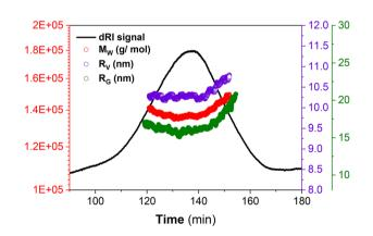
Fig. 4 ThFFF with triple detection for analysing  ${\rm PS_{102}-PEO_{34}}$  at  $\Delta T$  80 °C.
