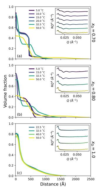
Fig. 5 Polymer volume fraction profiles of a PNIPAM brush derived by neutron reflectometry in various solvent compositions of increasing as a function of temperature: (a)  $x_D = 0.70$ , (b) 0.80 and (c) 1.0 (pure DMSO). Inset presents corresponding reflectivity and models.
