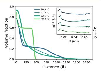
Fig. 2 Polymer volume fraction profiles of a PNIPAM brush as a function of temperature in  $D_2O$ . Thicker curves represent the VF profiles corresponding to the most swollen, partially collapsed and most collapsed structures. Inset presents corresponding reflectivity and models.
