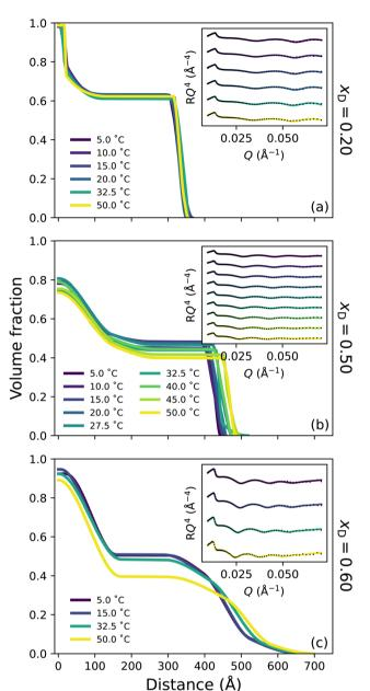
**Fig. 4** Polymer volume fraction profiles of a PNIPAM brush derived by neutron reflectometry in various solvent compositions of increasing  $x_{\rm D}$  as a function of temperature: (a)  $x_{\rm D}$  = 0.20, (b) 0.50 and (c) 0.60. Inset presents corresponding reflectivity and models.
