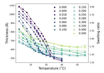
Fig. 1 Ellipsometry determined thickness and swelling ratio of a PNIPAM brush as a function of  $x_D$  and temperature. Circle symbols ( $\bullet$ ) denote solvent compositions where a clear thermotransition is observed; crosses (x) denote compositions with a severely suppressed thermotransition.
