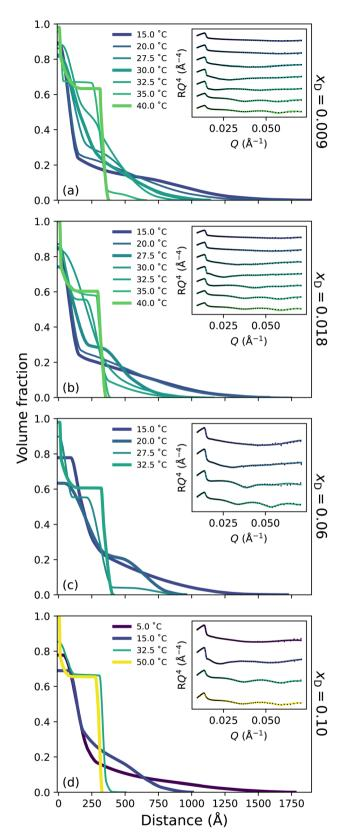
Fig. 3 Polymer volume fraction profiles of a PNIPAM brush as a function of temperature in (a)  $x_{\rm D}=0.009$ , (b) 0.018, (c) 0.06 and (d) 0.10. Thicker curves represent the VF profiles corresponding to the most swollen, partially collapsed and most collapsed structures.
