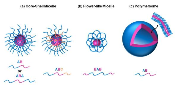
Fig. 5 Self-assembled structures adopted by amphiphilic block copolymers: (a) core-shell micelles by the AB, ABA, and ABC architectures, (b) flower-like micelles by the BAB architecture, and (c) polymersomes by the AB architecture. Blue and purple represent the hydrophilic and hydrophobic blocks, respectively, while when a second hydrophilic block is present, this is shown in orange. In the self-assembled structures, the compact hydrophobic part is represented by purple spheres.
