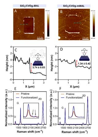
Fig. 3 (A and B) AFM scratching images and (C and D) height profiles of SiO<sub>2</sub>/CVDg-MAL (A and C) and SiO<sub>2</sub>/CVDg-mMAL (B and D). (E and F) Raman spectra of SiO<sub>2</sub>/CVDg-MAL (E) and SiO<sub>2</sub>/CVDg-mMAL (F) before and after the reaction
