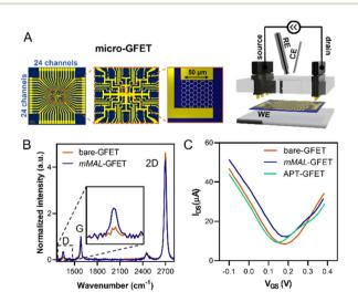
Fig. 5 Micro-GFET electrochemical functionalisation characterisation. (A) Schematic of the micro-GFET device and electrochemical setup. (B) Raman spectra of the pristine bare-GFFT and mMAI -GFFT (C) Transfer curves recorded on the micro-GFET recorded after each step of functionalisation.
