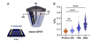
Fig. 4 Electrochemical functionalisation of the macro-GFET. (A) Schematic of the macro-GFET and set up for the electrochemical reduction. (B) Ratio between the intensity of D band and the intensity of G band of the Raman spectra recorded on pristine (orange) and functionalized (shading blues) graphenes by applying increasing CA time.
