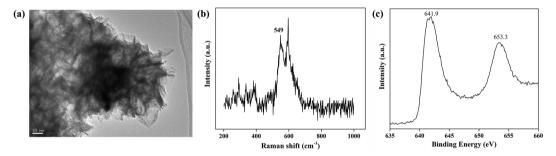
Fig. 6 (a) TEM image, (b) Raman spectrum and (c) XPS of MnO<sub>2</sub> nanosheets.
