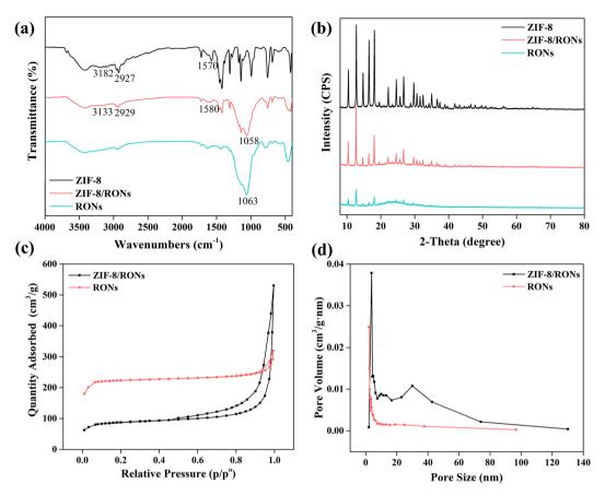
Fig. 3 (a) FT-IR spectra, (b) XRD curves, (c) N<sub>2</sub> extraction-desorption isotherms, (d) pore size of ZIF-8/RONs and RONs.
