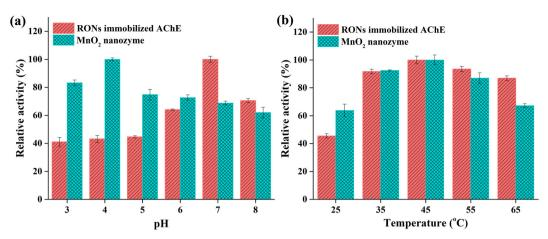
Fig. 7 (a) pH stability and (b) thermal stability of RONs immobilized AChE and MnO<sub>2</sub> nanozyme.
