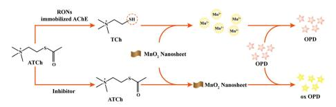
Fig. 1 Schematic of the assay of RONs immobilized AChE coupled with MnO<sub>2</sub> nanosheets for its inhibitor screening
