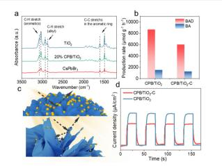
Fig. 7 (a) FTIR spectra of 20%CPB/TiO<sub>2</sub>, TiO<sub>2</sub> and CsPbBr<sub>3</sub> after adsorption of saturated toluene. (b) Photoactivity comparison between CPB/ TiO<sub>2</sub> and CPB/TiO<sub>2</sub>-C. (c) Schematic diagram of light absorption over CPB/TiO<sub>2</sub> and CPB/TiO<sub>2</sub>-C. (d) Transient photocurrent responses of CPB/TiO2 and CPB/TiO2-C.
