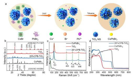
Fig. 1 (a) Schematic diagram of the synthesis of 3D nanoflower-shaped CPB/TiO<sub>2</sub> heterostructure. (b) XRD patterns, (c) Raman spectra, and (d) UVvis DRS spectra of CsPbBr<sub>3</sub>, CPB/TiO<sub>2</sub> and TiO<sub>2</sub>.
