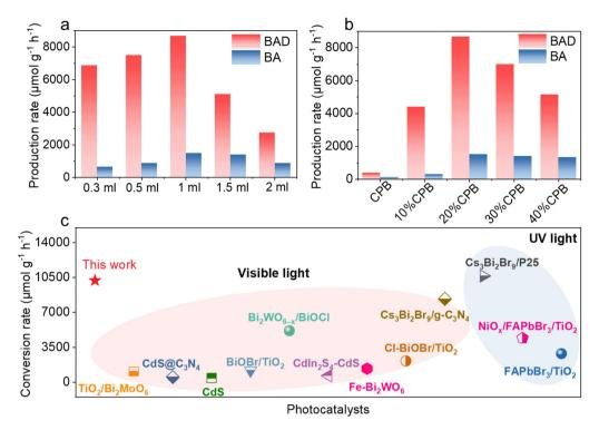
Fig. 5 (a) Photocatalytic oxidation of toluene with different toluene amounts in acetonitrile solvent over 20%CPB/TiO<sub>2</sub>. The total volume is 3 ml. (b) Photocatalytic oxidation of toluene over blank TiO2, CPB/TiO2 composite and blank CsPbBr3. (c) Performance comparison with reported photocatalysts for UV and visible-light-driven selective oxidation of toluene.
