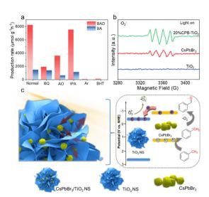
**Fig. 8** (a) Photocatalytic toluene oxidation in the absence or presence of various radical scavengers. (b) EPR spectra of DMPO-'O<sub>2</sub>-'. (c) Schematic illustration of the proposed mechanism of photocatalytic oxidation of toluene over the CPB/TiO<sub>2</sub> composite.
