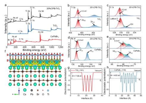
Fig. 4 XPS spectra of CsPbBr<sub>3</sub>, TiO<sub>2</sub> and 20%CPB/TiO<sub>2</sub>: (a) survey, (b) Ti 2p, (c) O 1s, (d) Pb 4f and (e) Br 3d. (f) Charge density differences in the CPB/TiO<sub>2</sub> composite. (g and h) The work functions of blank TiO<sub>2</sub> and CsPbBr<sub>3</sub>.
