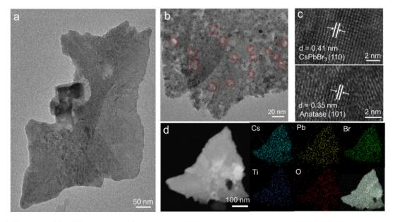
Fig. 3 (a and b) TEM images, (c) HRTEM image, and (d) corresponding EDS elemental mapping images of 20%CPB/TiO<sub>2</sub>.
