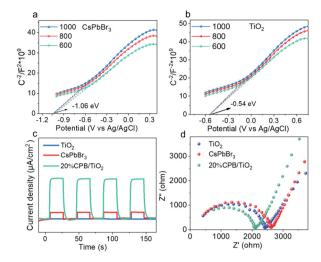
Fig. 6 (a and b) M-S plots of CsPbBr<sub>3</sub> and TiO<sub>2</sub>. (c) Transient photocurrent responses, and (d) EIS Nyquist plots of blank TiO2, CsPbBr3 and the CPB/TiO<sub>2</sub> composite.
