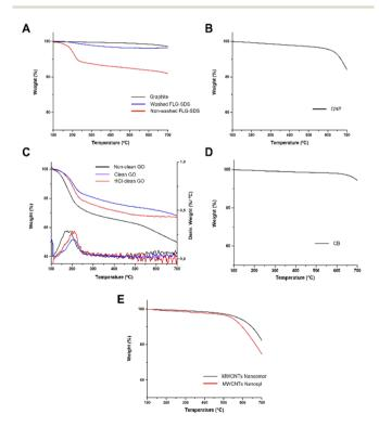
Fig. 2 Thermogravimetric analyses (TGA) of non-washed FLG-SDS and washed FLG-SDS (A), GNP (B), research-grade GO (C), CB (D) and MWCNTs NanoAmor and Nanocyl (E).
