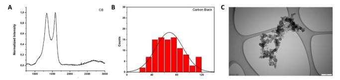
Fig. 5 Physico-chemical characterization of carbon black (CB). (A) Raman spectrum; (B) lateral dimension distribution; and (C) representative TEM image. Scale bar: 200 nm.
