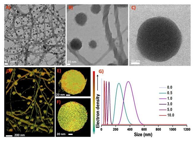
Fig. 4 TEM images showing the self-assembled superhelices and spheres NCA-1.0. Magnified TEM images are shown in A–C. (D) Electron tomography (ET) reconstruction of NCA-1.0. (E) and (F) are the 3D reconstructed structure of the  $Ag_{14}$  NC assembled sphere and its cross-sectional view. (G) DLS measurements show variation in size of  $[Ag_{14}(NT)_7(DPPH)_2Cl_2]^+$  NCs with the addition of different molar ratios of DPPH ligands.
