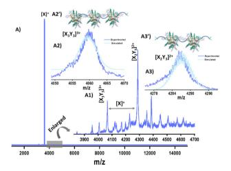
Fig. 5 (A) ESI MS showing the supramolecular adducts in NCA-1.0. (A1) Enlarged view of the same. (A2) The experimental and theoretical isotopic patterns of  $[X_3Y_3]^{3+}$ . (A2') Schematic representation of  $[X_3Y_3]^{3+}$ . (A3) The experimental and theoretical isotopic patterns of  $[X_2Y_3]^{2+}$ . (A3') Schematic representation of  $[X_3Y_3]^{2+}$ . (X =  $[Ag_{14}(NT)_7(DPPH)_2Cl_2]$ ; Y = DPPH). Color codes: grey, Ag; blue/sea green, C; yellow, S; orange, P; green, Cl; white, H.
