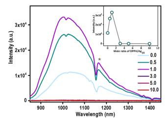
Fig. 6 Variation of PL trend of [Ag<sub>14</sub>(NT)<sub>7</sub>(DPPH)<sub>2</sub>Cl<sub>2</sub>]<sup>+</sup> NCs with the addition of different mole ratios of DPPH ligand (the star denotes the solvent-induced structuration). Inset shows the variation of PL intensity at 1035 nm with a different mole ratio of DPPH ligand.
