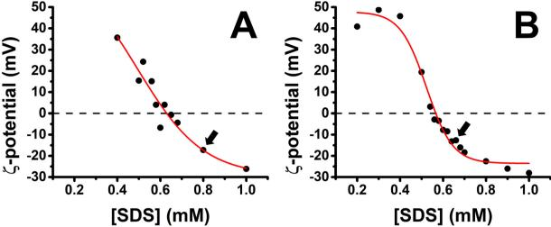
Fig. 2 Variation of the ζ-potential of (A) PLL/SDS (reproduced from ref. 27) and (B) PLA/SDS aggregates as a function of the concentration of SDS. The black circles represent the experimental data points and the red line a sigmoidal fit. The black dashed lines indicate neutral charge. The standard error in the ζ-potential values was found to be around 10%, smaller than the symbol size. Black arrows indicate the concentrations used to create
