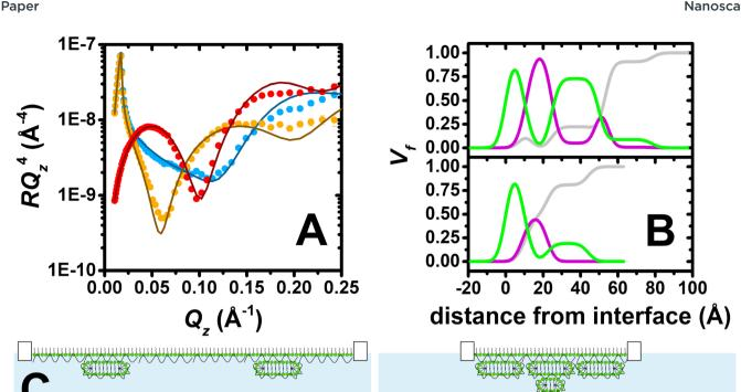
Fig. 3 (A) Neutron reflectivity profiles of a PLL/SDS film at a 4.5:1 compression ratio for d-SDS/ACMW (red circles), d-SDS/D<sub>2</sub>O (blue circles) and h-SDS/D<sub>2</sub>O (orange circles) contrasts. The continuous lines show the model fits. (B) Volume fraction profiles of SDS (green), solvent (grey) and PLL (purple) of PLL/SDS films at 4.5:1 (top) and 2:1 (bottom) compression ratios. (C) Schematic illustrations of the structures of PLL/SDS films using 2:1 and 4.5:1 compression ratios
