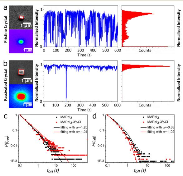
Fig. 3 SEM and PL images, PL intensity time trajectories (10 min, 100 ms bin time) and corresponding histograms of single MAPbI<sub>3</sub> crystals (a) before and (b) after the 3% MACl post-treatment, respectively. In the PL images, purple to red colors based on the rainbow sequence represent gradually higher intensities. Normalized probability distributions of the duration of (c) ON times and (d) OFF times of MAPbI<sub>3</sub> NCs with 0, 3%Cl surface treatment.
