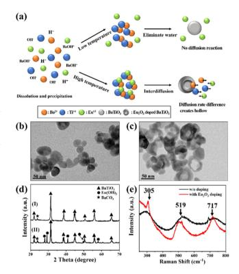
Fig. 1 (a) Schematic representation of the mechanism of formation of hollow nanoparticles through the Kirkendall effect. (b and c) TEM images of the BaTiO<sub>3</sub> nanoparticles prepared (b) without and (c) with Eu<sub>2</sub>O<sub>3</sub> doping. (d) XRD patterns of the BaTiO<sub>3</sub> nanoparticles prepared (I) without and (II) with Eu<sub>2</sub>O<sub>3</sub> doping. (e) Raman spectra of the BaTiO<sub>3</sub> nanoparticles prepared with and without Eu<sub>2</sub>O<sub>3</sub> doping.
