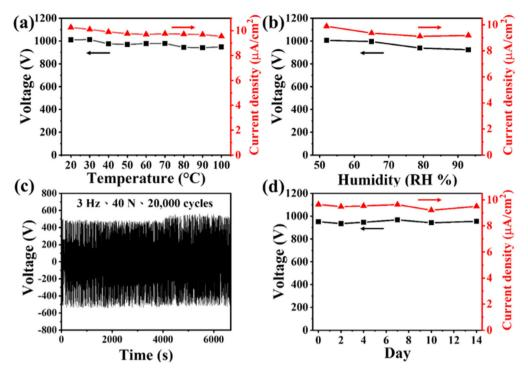
Fig. 4 Electrical output of the 10 wt% Eu<sub>2</sub>O<sub>3</sub>-BaTiO<sub>3</sub>/PVDF-HFP electrospun-nanofiber TENG (a) at various temperatures, (b) at various humidities, (a) during long-term cycling, and (d) during stability testing.
