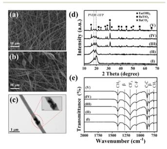
Fig. 2 (a and b) SEM images of electrospun (a) pristine PVDF-HFP nanofibers and (b) 10 wt%  $Eu_2O_3$ -BaTiO<sub>3</sub>/PVDF-HFP nanofibers. (c) TEM image of an electrospun  $Eu_2O_3$ -BaTiO<sub>3</sub>/PVDF-HFP nanofiber. (d) XRD patterns and (e) FTIR spectra of the (I) 0, (II) 1, (III) 5, (IV) 10, and (V) 15 wt%  $Eu_2O_3$ -BaTiO<sub>3</sub>/PVDF-HFP nanofibers.
