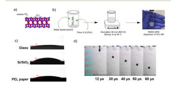
Fig. 1 (a) Structure of  $TiO_2$ -NS; (b) schematic of the  $TiO_2$ -NS ink formulation process; (c) droplet jetting sequence observed by the Dimatix printer camera; and (d) contact angles of the  $TiO_2$ -NS ink on glass, Si/SiO<sub>2</sub> and PEL-P60 paper substrates, respectively.
