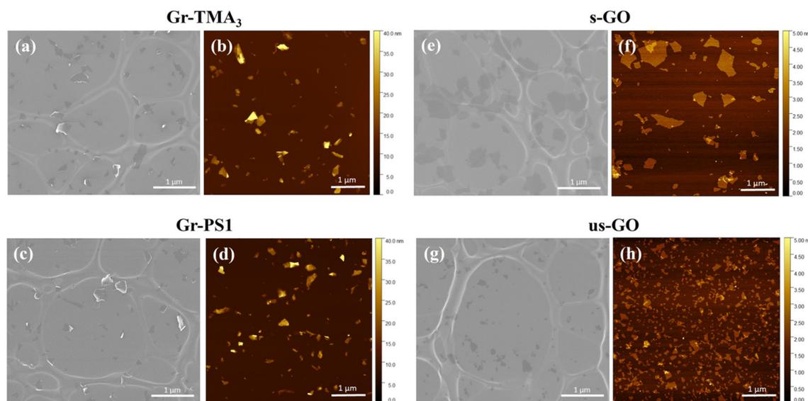
**Fig. 1** Physicochemical characterisation of (a and b) Gr-TMA<sub>3</sub>, (c and d) Gr-PS1, (e and f) s-GO and (g and h) us-GO: (a, c, e and g) electron and (b, d, f and h) AFM micrographs were obtained for lateral dimension and thickness measurements, respectively.
