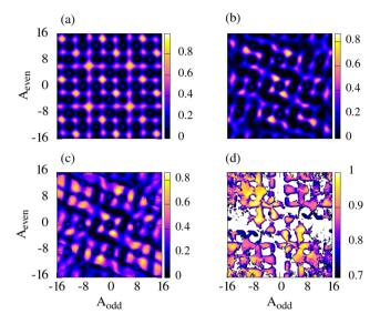
Fig. 6 Fidelity map of the  $\mathcal{P}_{ab}^-$  gate as a function of the pulse areas (in units of  $\pi$ ) in a 3-qubit system. (a) JP scheme with  ${c_k}^2=0.1$  for all pulses. (b) SOP with  $b^2=0.1$  and  ${c_k}^2=0.1$ . (c) SOP with optimized  $c_k$  imposing symmetric and orthogonal conditions in qubits a and b. (d) Fidelity performing at optimized  $a_k$  and  $b_k$  for  ${c_k}^2=0.1$ , imposing symmetric conditions.
