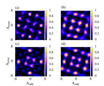
Fig. 7 Fidelity map for M-pulse sequence extensions of the SOP with (a) M = 2, (b) M = 3, (c) M = 4, (d) M = 5. We fixed  $b^2 = 0.1$  in all cases.
