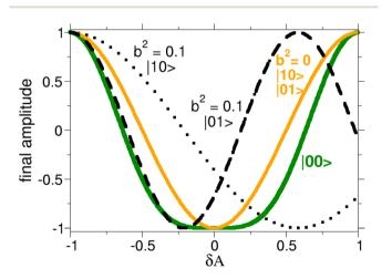
Fig. 2 Dependence of the final amplitude of the starting state (|00),  $|01\rangle$  and  $|10\rangle$ ) on deviations from  $\pi$  in the pulse areas of odd pulses  $(\delta A_1 = \delta A_3 = \delta A)$ , and of  $2\pi$  in the second pulse  $(\delta A_2 = 2\delta A)$ , for different geometrical factors.
