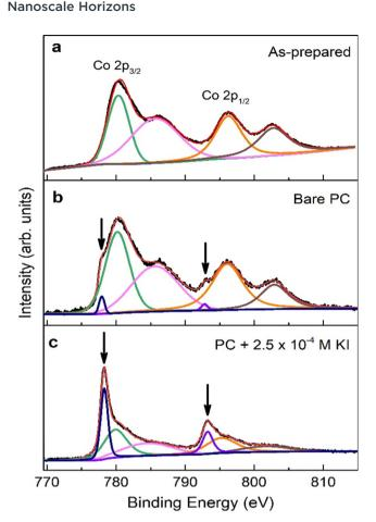
Fig. 5 X-ray photoelectron spectra of Co  $2p_{1/2}$  and Co  $2p_{3/2}$  for (a) asprepared, (b) treated in bare PC and (c) PC +  $2.5 \times 10^{-4}$  M KI samples. The downward arrows point to the Co  $2p_{3/2}$  and Co  $2p_{1/2}$  peaks of metallic Co (in blue and purple in (b) and (c)). Additionally, green and orange correspond to Co<sup>2+</sup>, and pink and brown to Co<sup>3+</sup>. Solid black lines are experimental data, whereas solid red lines refer to fitting spectra.
