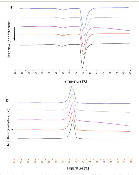
Fig. 3 The DSC (a) heating, and (b) cooling curves of DPPC: DPPG (9:1 molar ratio) at 0 (black line), 0.1 (red line), 0.2 (purple line), 0.5 (green line) and 1 mg mL $^{-1}$  (blue line) of **f-CNHs**.
