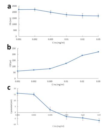
Fig. 5 (a) Hydrodynamic diameter and (b) scattering intensity over time, and (c) ζ-potential versus insulin concentration, of f-CNH:insulin complexes
