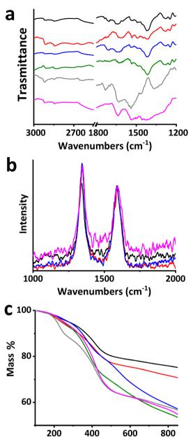
Fig. 1 (a) ATR-IR spectra, (b) Raman spectra (514 nm), and (c) thermogravimetric analysis graphs, obtained under a nitrogen atmosphere, of materials 5 (black), 6 (red), 7 (blue), 8 (green), and 9 (grey) and f-CNHs (pink)
