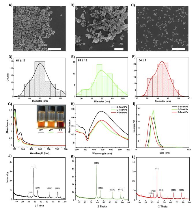
Fig. 1 The characterization of the synthesized TeaNPs: SEM pictures of (A) B-TeaNPs, (B) G-TeaNPs, and (C) R-TeaNPs. Scale bars correspond to 500 nm. Size distributions of (D) B-TeaNPs, (E) G-TeaNPs, and (F) R-TeaNPs; (G) UV-vis spectra of tea extracts, (H) UV-vis spectra of TeaNPs, and the spectra were normalized. (I) DLS size estimation of TeaNPs. The XRD diffractograms of (J) B-TeaNPs, (K) G-TeaNPs, and (L) R-TeaNPs.
