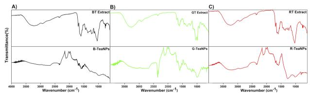
Fig. 2 FTIR spectra of (A) black tea extract and B-TeaNPs; (B) green tea extract and G-TeaNPs; (C) red tea extract and R-TeaNPs. The top line on each graph marks 100% transmittance
