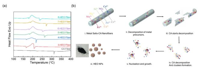
Fig. 2 (a) DSC of the fibers, and (b) proposed mechanism of HEO nanoparticles formation by converting the electrospun nanofibers *via* low-temperature annealing in air and the accomplished powder. A digital photograph of the as-synthesized HEO NPs.
