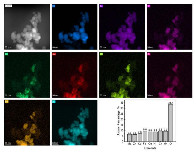
STEM and EDS mapping of 8-HEO NPsEDS elemental mapping of all eight individual metal elements and oxygen.
