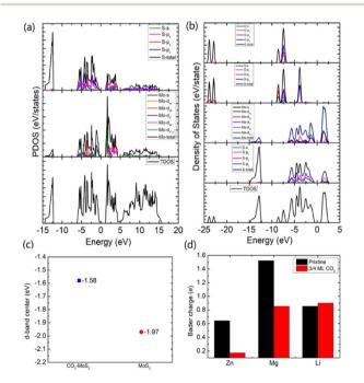
Fig. 5 The calculated projected density of states (PDOS) of the pristine MoS<sub>2</sub> (a) and CO<sub>2</sub> intercalated MoS<sub>2</sub> (b). (c) The calculated Mo d-band center with respective to the Fermi level (set to zero) of CO2 intercalated and pristine MoS2. (d) The calculated Bader charge of metal ions in the pristine and CO2 intercalated (3/4 ML) MoS2.
