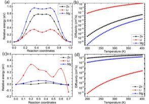
Fig. 2 The computed diffusion barriers (a) and (c) and diffusivities (b) and (d) of metal Zn, Li, and Mg ions in pristine bilayer  $MoS_2$  and in bilayer  $MoS_2$  with an intercalating  $CO_2$  coverage of 3/4 ML, respectively.
