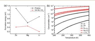
Fig. 3 The intercalation energies (a) and temperature-dependent concentration (b) of metal ions of Zn, Mg and Li in the pristine and modulated bilayer MoS<sub>2</sub> with an intercalating CO<sub>2</sub> coverage of 3/4 ML.
