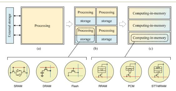
Fig. 2 The development of the computing structure. (a) von Neumann architecture. (b) Near-memory computing structure. (c) Computing-in-memory structure.
