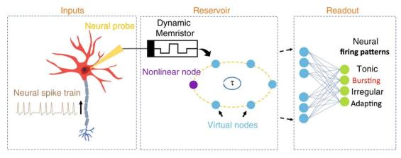
Schematic showing the concept of a memristor-based RC system for neural activity analysis
