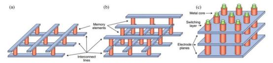
Fig. 4 RRAM across-array architecture and scaling.<sup>25</sup> (a) RRAM across-array structure with a single memory layer. (b) Horizontal stacked 3D across-array structure. (c) Vertical 3D across-array structure.
