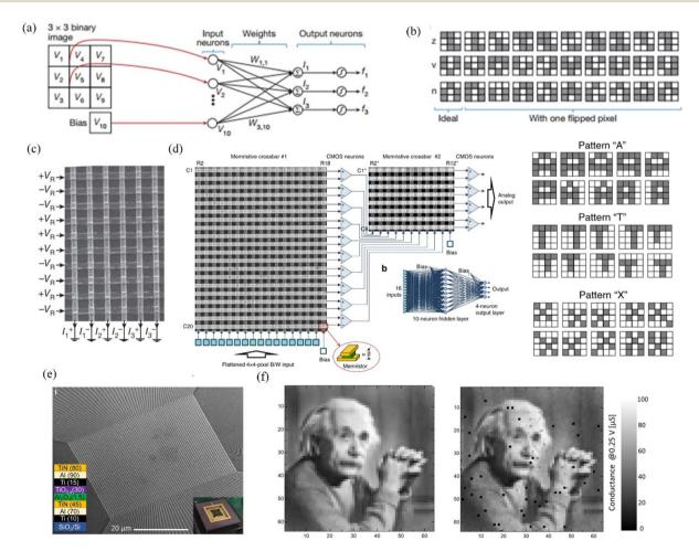
Fig. 8 Perceptron network based on RRAM. (a–c): Single-layer perceptron network. (a) Top-level description of the network. (b) The used input pattern set. (c)  $12 \times 12$  RRAM across-array circuit. (d–f): Multilayer perceptron network. (d) Double layer  $20 \times 20$  RRAM across-array circuit combined with the CMOS process. (e)  $64 \times 64$  RRAM passive across-array circuit. (f) Programming Einstein image to (e) with a 5% relative error.
