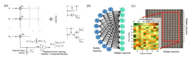
Fig. 9 Stochastic neural networks.<sup>52</sup> (a) Stochastic dot-product circuit and its applications in neurocomputing. (b) RRAM-based restricted Boltzmann machine. (c) A bipartite graph of the considered RBM network and its implementation (the red rectangle highlights the utilized area of a  $20 \times 20$  across-array).
