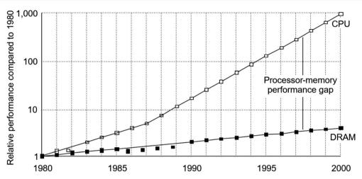
Fig. 1 Processor-memory performance gap
