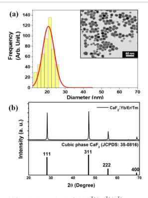
Fig. 4 (a) Size distribution for the  $CaF_2:Yb^{3+}/Tm^{3+}/Er^{3+}$  nanoparticles. The inset shows a TEM image of these nanoparticles. The bar size is 60 nm. (b) X-ray powder diffraction patterns of  $CaF_2:Yb^{3+}/Tm^{3+}/Er^{3+}$  nanoparticles (top) and the standard XRD pattern (bottom).
