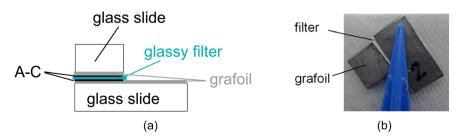
Fig. 2 (a) A cross section of the sample with grafoil coated active carbon (AC) electrodes and (b) a picture of the cover area ca,  $1.27 \times 1.27 \text{ cm}^2$ .
