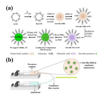
Fig. 1 (a) Stepwise representation of route to star-like PAA-b-PS diblock copolymer nanoreactor and the resulting PS-capped CsPbBrz nanocrystal. (b) Schematic diagram of dual flow/nano reactor apparatus.
