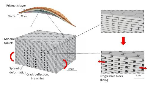
Fig. 1 Schematic of Nacre's brick-wall architecture and the prevailing toughening mechanisms. Reproduced from ref. 4 and 10 with permission from Springer Nature, copyright 2020, and the American Association for the Advancement of Science, copyright 2019.
