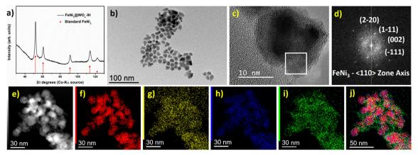
Fig. 6 FeNi<sub>3</sub>@W-IH NPs, (a) powder XRD pattern (ICDD: 00-038-0419, red vertical drop lines for standard FeNi<sub>3</sub>), (b) BF TEM micrograph, (c) HRTEM image and the corresponding FFT analysis (d) from the white square marked region, (e)–(j) STEM HAADF image and the respective STEM EDS elemental mapping shows Ni in red, O in yellow, Fe in blue, and W in green, and the overlap maps of W, Fe, and Ni.
