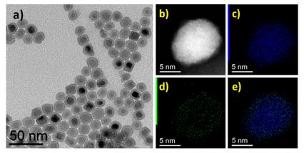
Fig. 2 Fe<sub>2.2</sub>C@Mo-TH NPs, (a) BF TEM image, (b) STEM-HAADF image and STEM-EDX mapping showing (c) Fe (blue), (d) Mo (green), and (e) overlap of Fe and Mo maps
