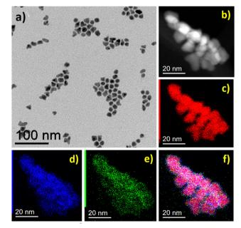
Fig. 1 FeNi<sub>3</sub>@Mo-TH NPs, (a) BF TEM image, (b) STEM-HAADF image and STEM-EDX mapping of the sample, (c) Ni (red), (d) Fe (blue), (e) Mo (green), and (f) overlap of Fe, Ni, and Mo maps.
