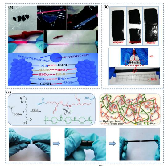
Fig. 8 (a) Self-healing of the obtained hydrogel and the illustration of the mechanism. <sup>136</sup> Reprinted from ref. 136 with permission. Copyright 2019 Royal Society of Chemistry. (b) Self-healing test of CNC-PANI/PVA hydrogels with a healing time of 30 s. Reprinted from ref. 153 with permission. Copyright 2020 Elsevier. (c) Diagrammatic illustration of the structure and characterization of the CPHs. Reprinted from ref. 168 with permission. Copyright 2021 John Wiley and Sons.
