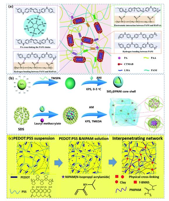
Fig. 6 (a) Hydrophobic association of the physically cross-linked PAAN hydrogels and the interactions within the gel. Reprinted from ref. 133 with permission. Copyright 2021 Royal Society of Chemistry. (b) The preparation of a SiO<sub>2</sub>@PANI-P(AM/LMA) hydrogel. Reprinted from ref. 135 with permission. Copyright 2021 Royal Society of Chemistry. (c) Fabrication process of f-BNNS/PEDOT:PSS/PNIPAM hydrogels. Reprinted from ref. 136 with permission. Copyright 2019 Royal Society of Chemistry.
