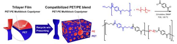
Fig. 6 Compatibilization of PET-PE multiblock copolymer and synthetic scheme for the preparation of PET-PE MBCP. Reproduced with permission from ref. 20. Copyright 2020 ACS Appl. Mater. Interfaces.
