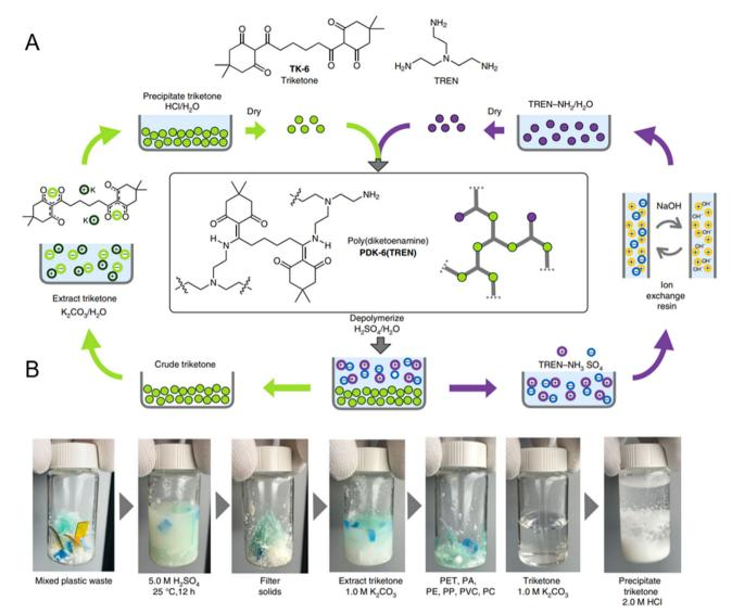
Fig. 13 (A) Mechanism for polydiketoenamine synthesis and depolymerization. (B) Polydiketoenamine based polymers can be extracted from a mixed plastic waste source to obtain pure triketone. Reproduced in part with permission from ref. 37. Copyright 2019 Nature Chem.
