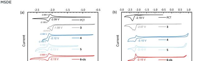
Fig. 3 Cyclic voltammograms of the macrocycles (a) in dimethylformamide (DMF) solution, and (b) in thin films dropcast onto the working electrode. The voltammograms were recorded using a glassy carbon working electrode, a platinum counter electrode, and a silver wire quasireference electrode (QRE) at a scan rate of  $0.1 \text{ V s}^{-1}$ .  $0.1 \text{ M } [n\text{-Bu}_4\text{N}]\text{PF}_6$  solutions in either DMF (solution) or acetonitrile (thin film) were used as the supporting electrolyte.
