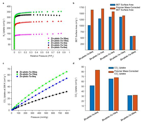
Fig. 4 N<sub>2</sub> (a) and CO<sub>2</sub> (c) gas sorption isotherms for a series of polyMOF-5 materials synthesized from pbdc-7a and x equivalents of free H<sub>2</sub>bdc linkers and a comparison of the polyMOFs' BET surface areas (b) and total CO2 uptake at 298 K and 1 atm (d). BET surface areas and CO2 uptake capacities corrected to only account for the mass contributing to the framework are shown in red.
