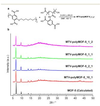
Fig. 5 (a) Synthesis of mixed polymer ligand polyMOFs MTVpolyMOF-5\_x\_y from x equivalents of pbdc-7a and y equivalents of pabdc-0a and (b) powder X-ray diffractogram of series of MTVpolyMOF-5\_x\_y.
