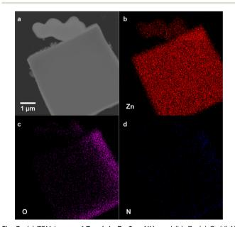
Fig. 3 (a) TEM image of Zn-pbdc-7a-2eq-NH<sub>2</sub> and (b), Zn (c) O, (d) N EDX elemental mapping of Zn-pbdc-7a-2eq-NH<sub>2</sub>, indicating incorporation of free bdc-NH2 ligand into polyMOF lattice.
