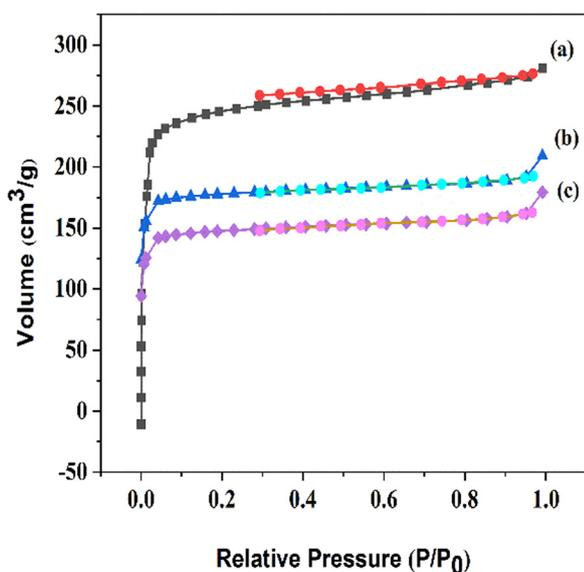
Fig. 2 N<sub>2</sub> adsorption-desorption isotherms of (a) MIL-68(In), (b) MIL-68(In)-malo, and (c) MIL-68(In)-PhDA.
