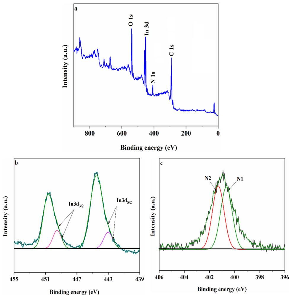
Fig. 1 Typical XPS survey spectra of MIL-68(In)-PhDA (a), In 3d spectra (b) and N 1s spectra (c) of MIL-68(In)-PhDA.
