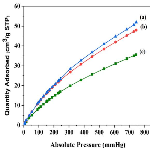
Fig. 3 CO<sub>2</sub> sorption isotherms of (a) MIL-68(In)-PhDA, (b) MIL-68(In)-malo, and (c) MIL-68(In) at 298 K.
