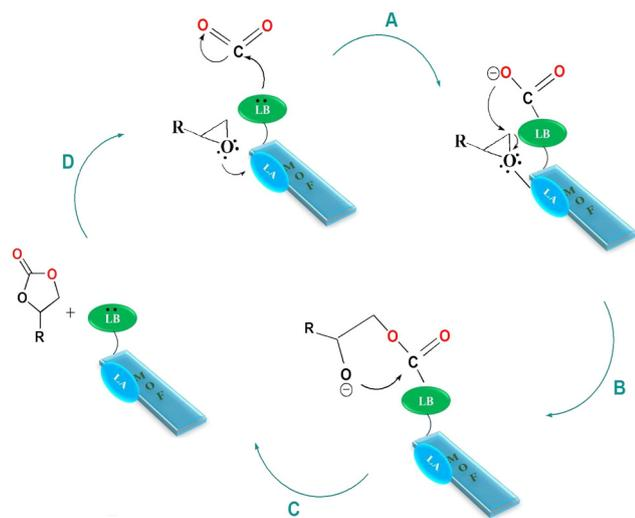
Scheme 2 Proposed mechanism for cycloaddition of CO<sub>2</sub> by modified MIL-68(In) catalyst. MOF: metal-organic framework, LA: Lewis acid, LB: Lewis base.
