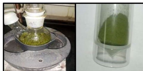
Fig. 1 Synthesis of PANI/Te nanocomposite.
