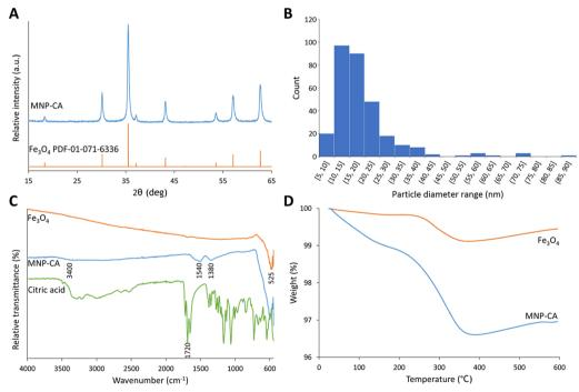
Fig. 2 (A) PXRD patterns of synthesised MNP-CA and pristine Fe<sub>x</sub>O<sub>4</sub> from the powder diffraction file database (PDF-01-071-6336).<sup>50</sup> (B) Histogram showing the size distribution of MNP-CA from TEM image analyses. (C) FTIR spectra for pristine Fe<sub>3</sub>O<sub>4</sub>, synthesised MNP-CA, and citric acid. (D) Graph showing weight loss on heating during TGA for pristine Fe<sub>3</sub>O<sub>4</sub> and synthesised MNP-CA.
