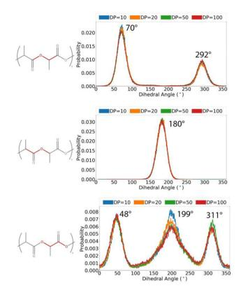
**Fig. 3** Distributions of key dihedral angles in the PLA backbone, for amorphous systems of varying chain lengths, calculated from a simulation at 298 K in the *NVT* ensemble.
