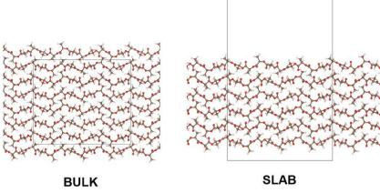
Fig. 1 Bulk and slab structures of crystalline PLLA.
