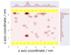
Fig. 8 A KDE plot demonstrating the probability density of locations occupied by molecular oxygen (red) and silicon atoms (yellow) in an oxygenated PLA/pyrophyllite system, with coordinates extracted from all frames across 20 duplicate simulations. Regions of darker red indicate coordinates which are occupied by oxygen for a longer period of time.
