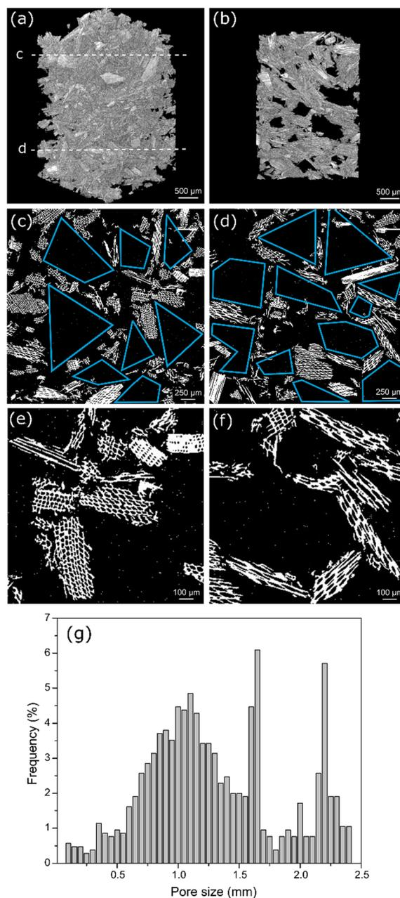
Fig. 3 Reconstructed  $\mu$ CT images of a wood foam prepared with a wood/PVA ratio of 3 showing (a and b) 3D-overview; (c and d) cross-sections from (a) with polyhedral cells highlighted in blue; (e and f) cross-sections showing the honeycomb structures of the wood cell wall; (g) pore size distribution from morphological segmentation. See video ESI,† for the 3D rendering of panel (a).
