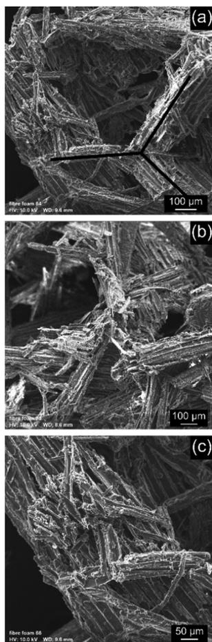
Fig. 4 SEM images of the wood foams exhibiting (a) cellular pores with milled wood assembled as a tetrahedral framework; (b) wood-PVA interlocked structures formed from milled wood with widths  $< 50 \mu\text{m}$ , (c) short milled wood particles ( $< 500 \mu\text{m}$  long) assembled along the surface of longer milled wood particles ( $> 800 \mu\text{m}$  long).
