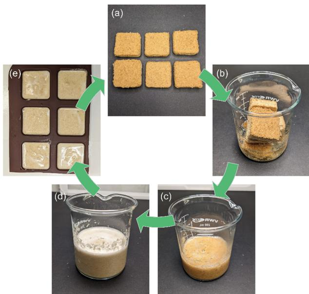
**Fig. 8** Re-foamability test showing (a) dried wood foams; (b) wood foams being soaked in water, (c) re-wetted and mixed wood foams forming a slurry that is indistinguishable from the original, (d) re-foamed wood slurry; (e) re-foamed wet wood foams in silicone molds prior to oven-drying – dried foams are also indistinguishable from the originals.
