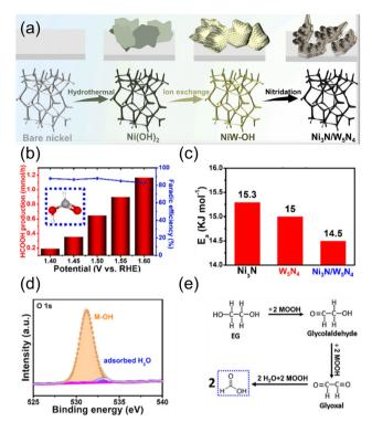
Fig. 9 (a) Schematic illustration of the formation Ni<sub>3</sub>N/W<sub>5</sub>N<sub>4</sub>. (b) Formate production rate and FE under different potentials. (c) E<sub>a</sub> value for the catalysts in DI water + plastics. (d) High-resolution XPS spectrum of O 1s (about Ni<sub>3</sub>N/W<sub>5</sub>N<sub>4</sub>). (e) The suggested reaction mechanism for the formate-selective EGOR. Reprinted with permission from ref. 72. Copyright 2022 Elsevier.
