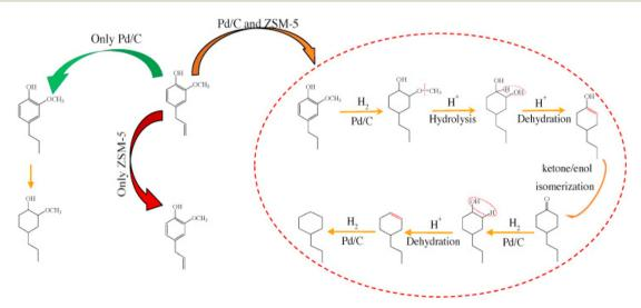
Fig. 12 Reaction pathways of eugenol to cyclohexanes over Pd/C and HZSM-5 in the aqueous phase. 85
