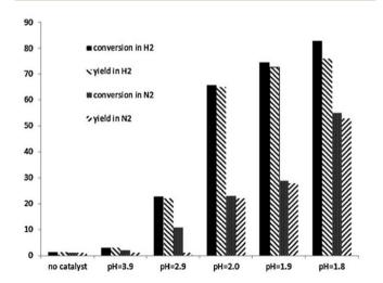
Fig. 6 Demethylation of guaiacol at 280 °C in aqueous HCl at different pH values. Both conversion of guaiacol and catechol yield after 3 hours are shown. Reactions were conducted either under a N2 or H2 atmosphere. Reproduced from ref. 72 with permission from Elsevier, copyright 2013.
