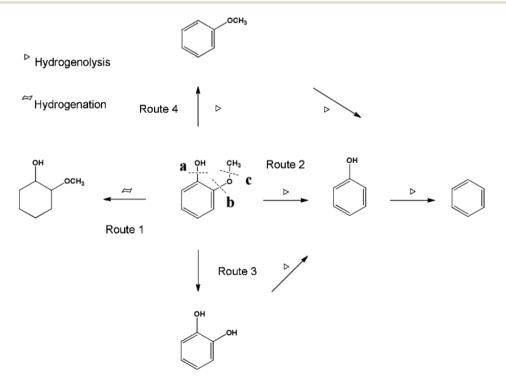
Fig. 13 The plausible reaction pathways for quaiacol conversion with metal/acid bifunctional catalysts in the aqueous phase. Reproduced from ref. 104 with permission from the Royal Society of Chemistry, copyright 2016.
