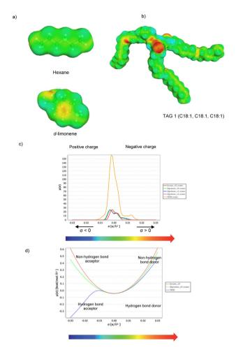
Fig. 3 Step calculation with COSMO-RS: (a) D-limonene and n-hexane  $\sigma$ -surface; (b) oleic acid triglyceride (TAG 1)  $\sigma$ -surface; (c) energies of local surface interactions between  $\sigma$ -profiles of TAG 1 and the two solvents; (d)  $\sigma$ -potentials of TAG 1 and solvents. [Reproduced from ref. 32 with kind permission from American Chemical Society, Copyright 2019].
